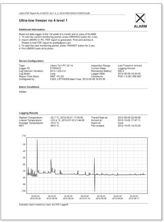
Electronic records are far superior to handwritten records and chart readouts. This example of a data logger report shows device settings, high, low and average temperatures, and more.
